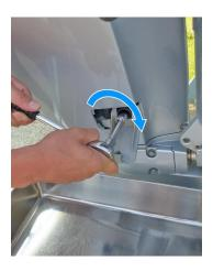
After draining the oil, install the drain bolt and new sealing washer, and tighten the bolt securely.
