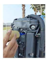
15. Pour a teaspoon of engine oil into all the spark plug holes to lubricate the inside of the cylinders.
