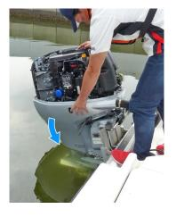
8. Tilt the outboard motor down.
