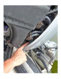
7. Clamp the drain tube on the front bracket clamp.
