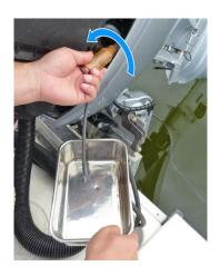
Loosen the vapor separator drain screw. Drain the petrol into the drain pan as it flows out of the drain tube.
