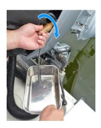
6. After draining, tighten the drain screw.
