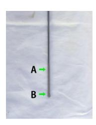
13. Check the oil level, insert the dipstick all the way to the engine then read the level. The oil level must be between the upper level (A) and lower level (B).
